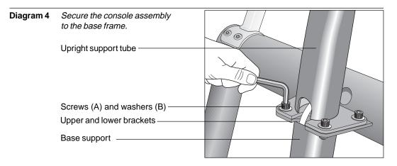
7. Secure the console assembly to the base frame support. Diagram 4. Place a washer (B) on each of 4 screws (A). Align the mounting holes and insert the screws through the upper and lower bracket. Use the hex key provided to alternately tighten each screws until all four screws are secure.
